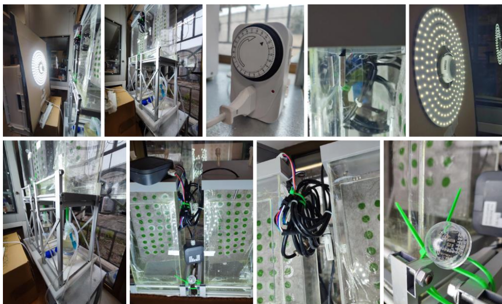
Figure 1. Laboratory-scale Twin Layers photobioreactor prototypes with sensors, polycarbonate discs and attached biomass.
